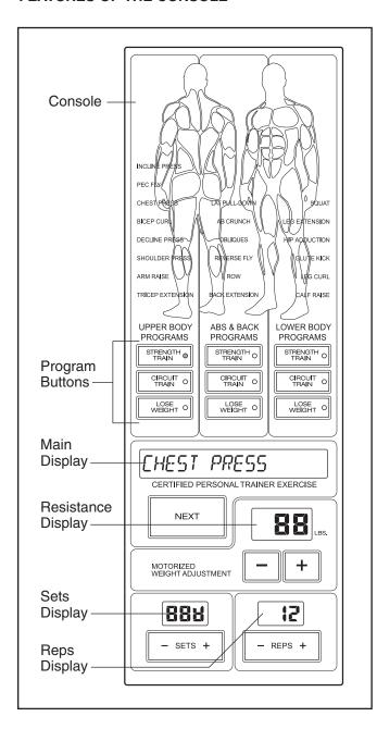
The heart of the resistance system is the digital resistance training console. The console offers both a manual mode and nine workout programs. When the manual mode is selected, the resistance setting can be changed with the touch of a button. When a program is selected, the console will guide you through an effective upper body, ab and back, or lower body workout.
